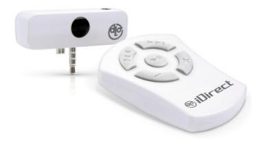
Like all of the IR-based remotes we tested, the iDirect provides very good range and reliability indoors—approximately 30 unobstructed feet—but does not function through walls or around corners.
